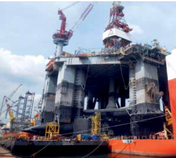
Diamond Offshore's semisubmersible drilling rig, Ocean Monarch, was onboard a heavy lift vessel, Dockwise White Marlin, for lower hull cleaning from 16 to 23 June 2015
