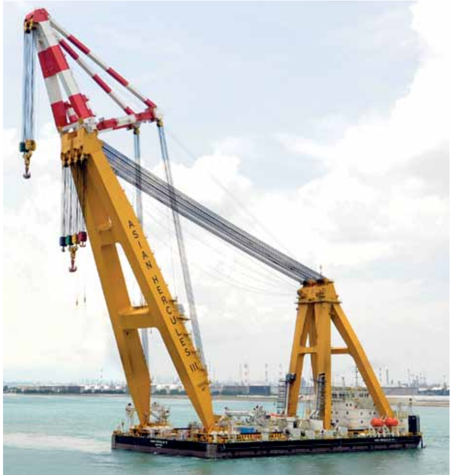
Asian Hercules III, the largest heavy-lift sheerlegs of its kind in the world, can perform single lifts of up to 5,000 tonnes
