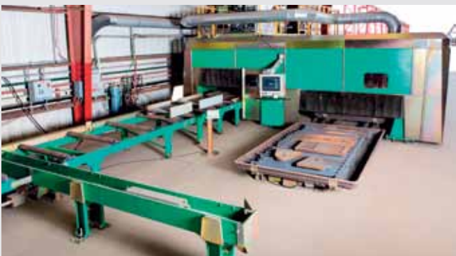
With the Steel Pro 900 2D/3D plasma cutting machine, one person is able to complete in 20 minutes what takes a crew of two approximately five hours for the same job
