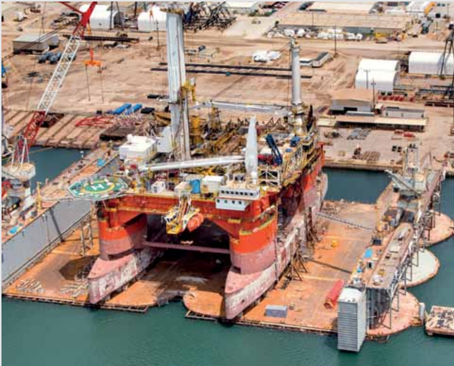
The yard leveraged its floating dry dock and floating crane to undertake thruster repairs and replacements on the Q4000 semi
